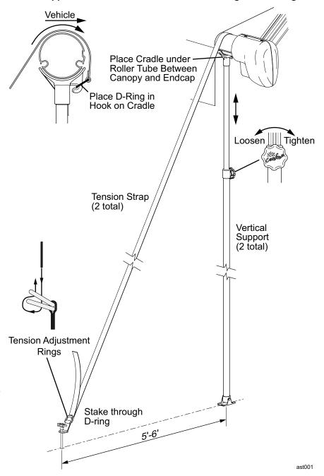
NOTICE | Always remove the supports before retracting the awning. Retracting the awning with the supports and tie-downs attached can damage the awning.
